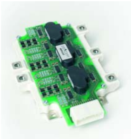
Figure 2: Six-channel Plug-and-Play driver 6SP0110T engineering sample made for Infineon HybridPACK™ 1
