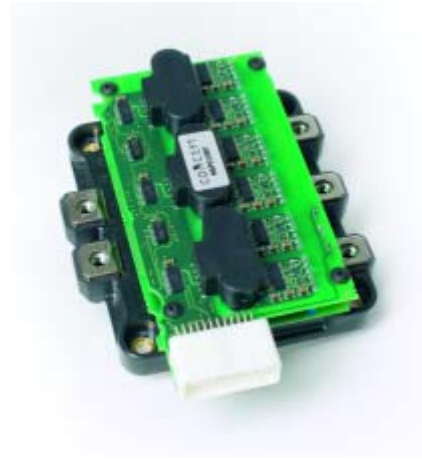
Figure 7: Six-channel Plug-and-Play driver 6SP0108T engineering sample made for Fuji 6MBI400VN-065V
