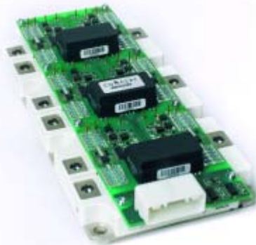
Figure 3: Six-channel Plug-and-Play driver 6SP0235T engineering sample made for Infineon HybridPACK™ 2
