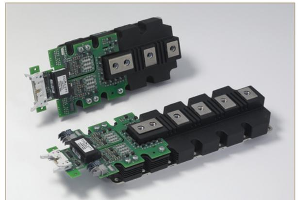
secondary-side gate driver chip has an integrated output stage for gate currents up to 6A. The output current can be increased to about 40A by simple means. The complete functionality of the DC/DC converter is integrated in the primary side interface chip. The user interface is compatible with all logic families from 3.3 to 15V.
