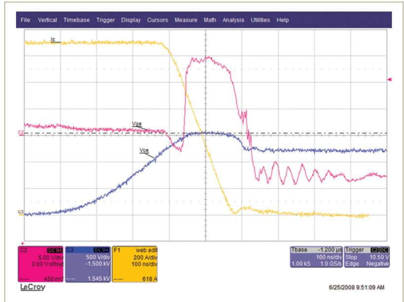
**Figure 3: Short-circuit turn-off of FF650R17IE4 at  $V_{DC} = 1200V$ ,  $L_s = 65nH$  and  $T_j = 150^\circ C$**
