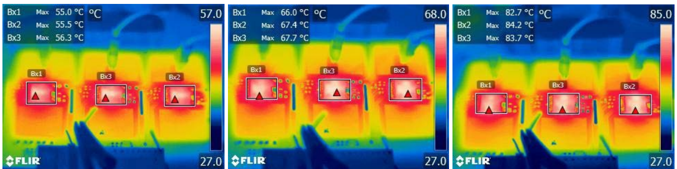
d) 100 W Inverter Output Power
