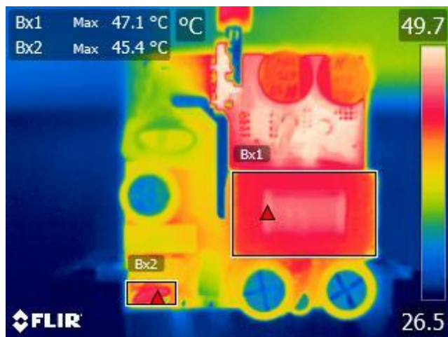
Figure 29 – Top Thermal Image. Bx1: Transformer, T1 = 47.1 °C. Bx2: Thermistor, RT1 = 45.4 °C.
