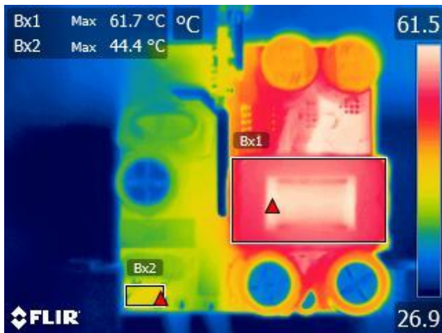
Figure 39 – Top Thermal Image. Bx1: Transformer, T1 = 61.7 °C. Bx2: Thermistor, RT1 = 44.4 °C.
