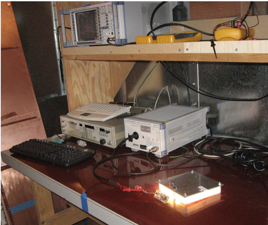
Figure 43 – Conducted Emissions Measurement Set-up.
