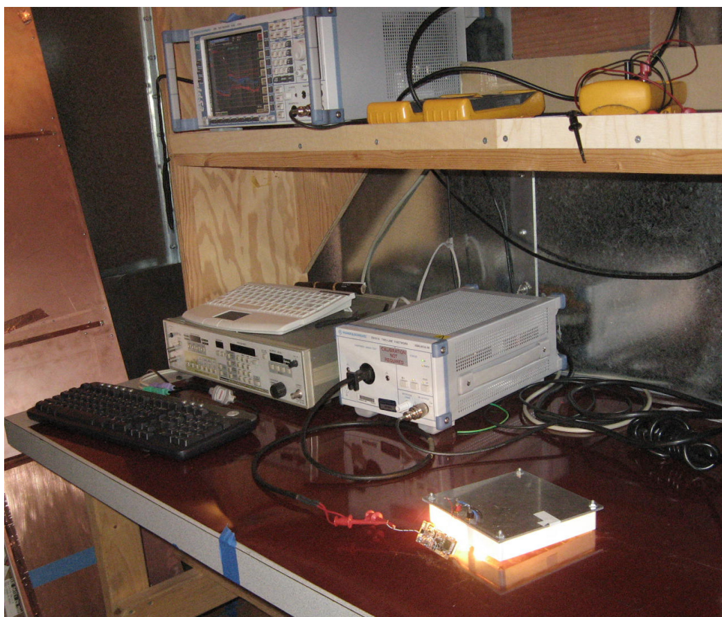
Figure 43 – Conducted Emissions Measurement Set-up.
