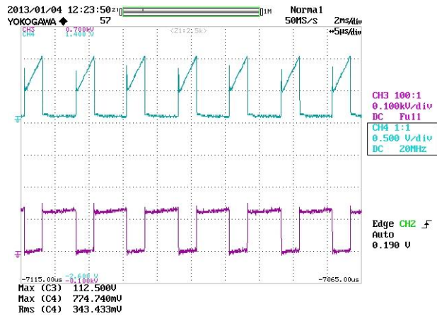
Figure 40 – 90 VAC, 60 Hz. Upper: I_{DRAIN} , 0.5 A / div. Lower: V_{DRAIN} , 100 V / div., 5 ns / div.
