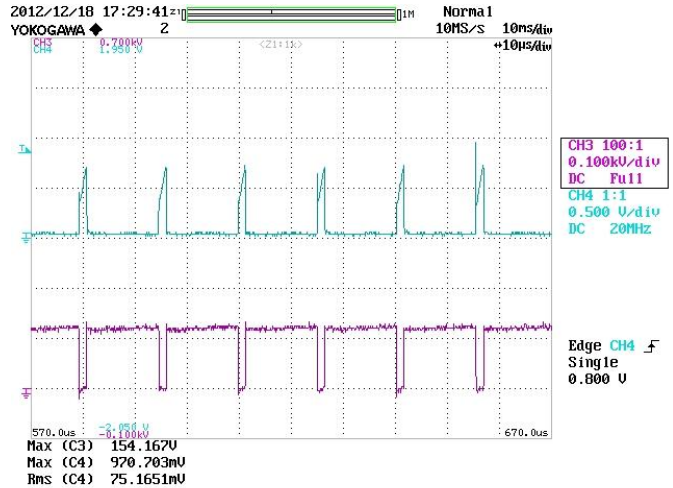
Figure 44 – 90 VAC, 60 Hz Start-up. Upper: I_{DRAIN} , 500 mA / div. Lower: V_{DRAIN} , 100 V, 10 \mu s / div.
