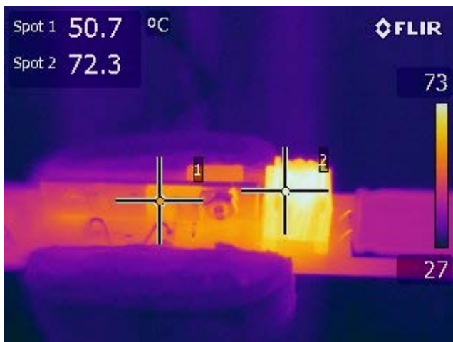
Figure 21 – 230 VAC, Full Load. Spot 1: LYT4213E. Spot 2: Transformer.
