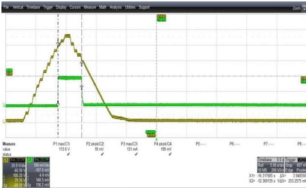
Figure 41 – DC_{IN} and 18 V Output Voltage. Waveform for Line UV Test. ( V_{UV+} : 100.3 V, V_{UV-} : 79.8 V) Upper: DC_{IN} , 20 V. Lower: 18 V, 10 V, 5 s / div.
