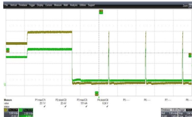
Figure 37 – Output Voltage Waveform. 90 VAC Input. Upper: 18 V, 5 V / div. Lower: 5 V, 2 V / 1 s div.
