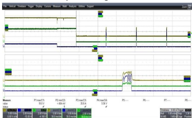
Figure 35 – Output Voltage and Current Waveforms. 90 VAC Input. Upper: 18 V, 5 V / div. Middle: 5 V, 2 V / div. Lower: I_{OUT} , 5 A, 1 s, 50 ms / div.
