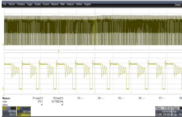
Figure 25 – Drain Voltage Waveforms. 265 VAC Input, Full Load, (574 V MAX ). V DRAIN , 100 V, 1 ms, 20 μs / div.
