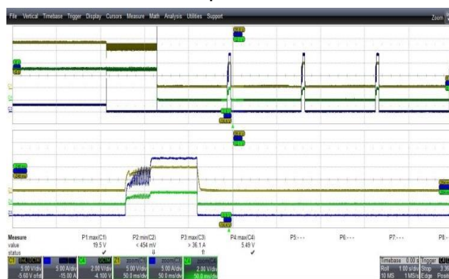
Figure 36 – Output Voltage and Current Waveforms. 265 VAC Input. Upper: 18 V, 5 V / div. Middle: 5 V, 2 V / div. Lower: I_{OUT} , 5 A, 1 s, 50 ms / div.
