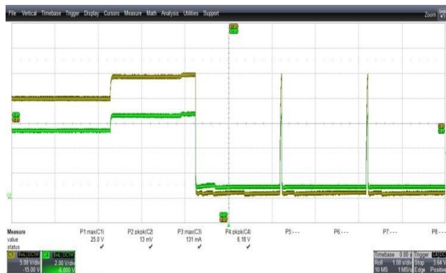
Figure 38 – Output Voltage Waveform. 265 VAC Input. Upper: 18 V, 5 V / div. Lower: 5 V, 2 V / 1 s div.
