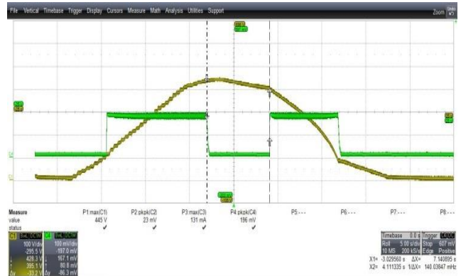
Figure 42 – DC_{IN} and 18 V Output Voltage. Waveform for Line OV Test. ( V_{OV-} : 428.3 V, V_{OV+} : 395.1 V). Upper: DC_{IN} , 20 V. Lower: 18 V, 10 V, 5 s / div.
