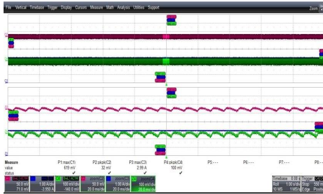
Figure 45 – Output Ripple Voltage Waveforms. 90 VAC Input. 3 A on 5 V and 1.4 A on 18 V. Upper: 5 V, 50 mV / div. Lower: 18 V, 100 mV, 20 ms / div.
