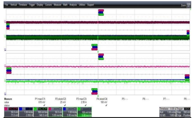
Figure 46 – Output Ripple Voltage Waveforms. 265 VAC Input. 3 A on 5 V and 1.4 A on 18 V. Upper: 5 V, 50 mV / div. Lower: 18 V, 100 mV, 20 ms / div.
