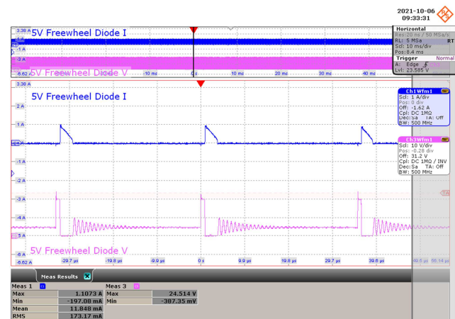
Figure 97 – 265 VAC 50 Hz. CH1: I_{5V\_Diode} , 1 A / div., 10 ms / div. CH3: V_{5V\_Diode} , 10 V / div., 10 ms / div. Zoom: 10 \mu s / div. PIV = 24.514 V, I_{D(MEAN)} = 0.011 A.
