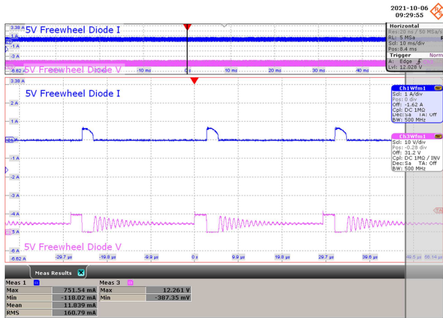
Figure 94 – 90 VAC 60 Hz. CH1: I_{5V\_Diode} , 1 A / div., 10 ms / div. CH3: V_{5V\_Diode} , 10 V / div., 10 ms / div. Zoom: 10 \mu s / div. PIV = 12.261 V, I_{D(MEAN)} = 0.011 A.
