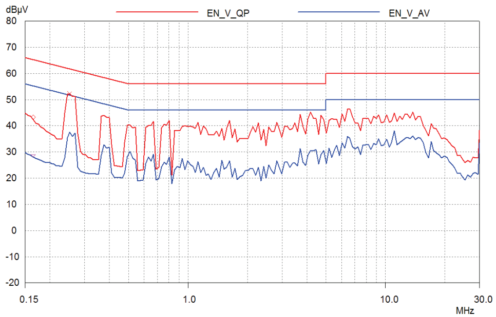
Figure 45 – Conducted EMI at 230 VAC 60 Hz, Full Load, and Output Return Connected to Ground.
