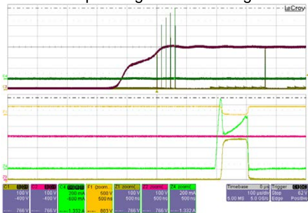
Figure 26 – 265 VAC / 50 Hz Start-up. Ch1, Z1: SOURCE Pin to Ground; 100 V / div. Ch2, Z2: Bulk Input; 100 V / div. Ch4, Z4: I_{DRAIN} ; 0.2 A / div. Time Scale: 100 \mu s / div. F1: V_{DS} ; 100 V / div. Zoom Time Scale: 500 ns / div.
